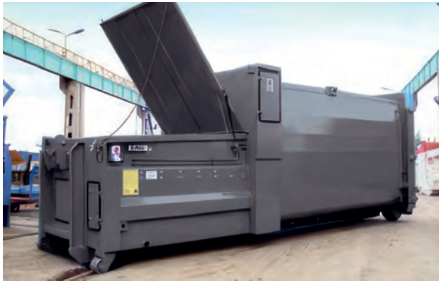
Ground-level feed opening with lockable lid
