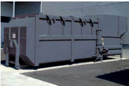
Wall-connected feed hopper
